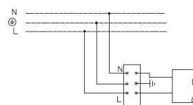
2. Mains connection scheme for luminaire with 1-10V regulated control gear.
