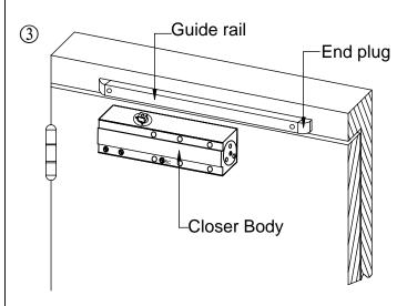
Mount guide rail on the door frame, and screw it tightly after inserting the slider and end plugs.
