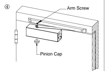
Attach the main arm to spindle and screw it tightly. Snap pinion cap over spindle on the bottom of closer body.
