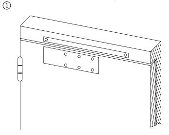
Mark 4 holes on door for closer and 2 holes on frame face for guide rail.
