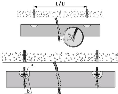
3. Attach the body to bearing surface with hardware kit into pre-made holes.
