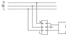
2. Mains connection scheme for luminaire with MS motion sensor.
