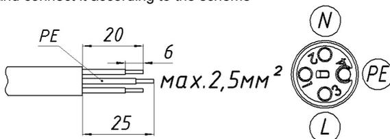
4. Lock wires with screws, assemble connector in reverse order. Bushings' tightening torque 2.5 Nm.
