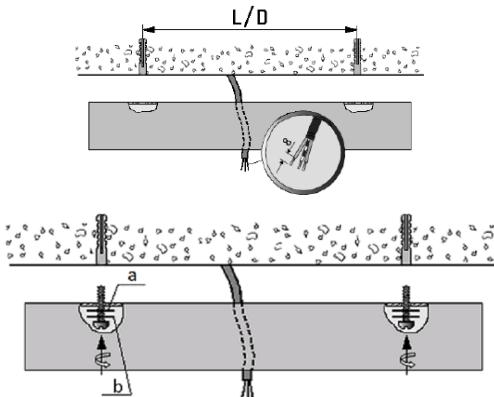
3. Connect mains cable to terminals according to polarity shown.
