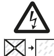
The light source contained in this luminaire shall only be replaced by the manufacturer or his service agent or a similar qualified person. In case of a malfunction, immediately unplug the luminaire from the mains supply.
