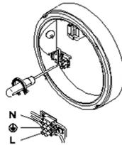
6. Install lamp with appropriate cap into base.
