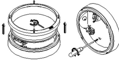
3. Put round (diameter 6.5 mm max) mains cable (length 180 mm at least) into luminaire's base through one of cable gland. Put mains cable through three openings in a row.
