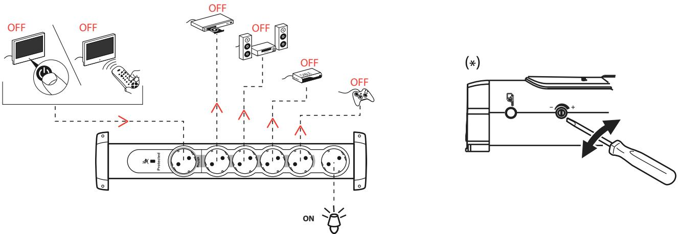
**GB** Connect your television or computer to the "MASTER" socket. When you turn off this device or put it on standby, power to the four controlled sockets is automatically cut off and any associated equipment plugged in to the unit is turned off.
