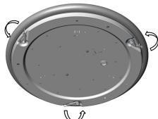
4. Put mains cable ( $\varnothing$  6-12 mm) into the luminaire's body through cable gland. Attach the body to bearing surface.
