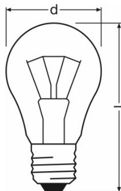
25 W 230 V E27, 40 W 230 V E27, 40 W 240 V E27, 60 W 230 V E27, 75 W 230 V E27
