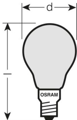
25 W 230 V E14, 40 W 230 V E14, 60 W 230 V E14, 40 W 240 V E14, 60 W 240 V E14
