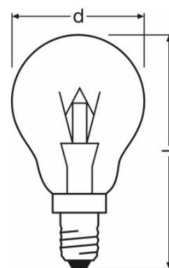
25 W 230 V E14, 40 W 230 V E14, 40 W 240 V E14, 60 W 230 V E14, 60 W 240 V E14
