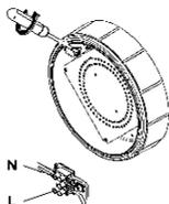
4. Place luminaire's base on bearing surface and lock it with appropriate hardware (no more 3.5mm in diameter) through plastic rings into mounting holes made beforehand.
