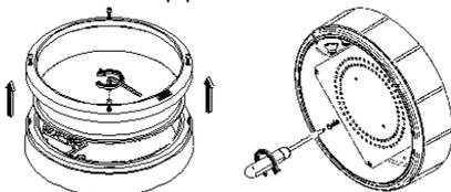
3. Put mains cable into luminaire's base through one of sealings, cable should have round profile, fix it with strain relief and connect to terminal block.
