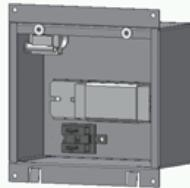
4. Connect mains cable to terminals according to polarity shown.
