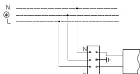
2. Mains connection scheme for luminaire with DALI regulated control gear.
