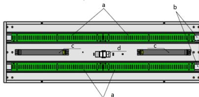
6. For the modification of Olympic LED80 it is necessary to adjust required angle of the lighting fixture installation (20, 40 degrees) by means of alignment of the working openings in brackets and fixation by M5 screws.
