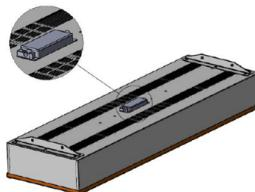
4. Align holes in brackets on the casing with ones in ceiling brackets by using M5 screws (included).
