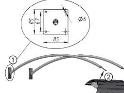
13.2. Place the brackets on bearing surface.
