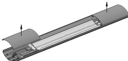
2. To prevent shrinkage of colorized decorative polymeric insert during operation it is necessary during line assembly to pull insert out of its slot at ~100-150 mm and carefully tuck it into slot beginning from luminaire edge. Cutting of the insert is prohibited.
