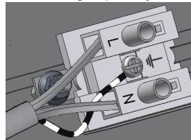
10. When building a line, mains cable is connected to terminals block of first luminaire (bear in mind maximal number of luminaires in a line). Next, luminaires' terminal blocks are interconnected with short cable following the polarity.
