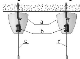
6. Installation directly on mounting surface (on fig. a-bushing, b-slider).
