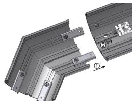
8. Attach the luminaire to prepared pendants. Next luminaire, with joining or angle aluminum brackets on it, should be joined with previously installed one, making line of luminaries.
