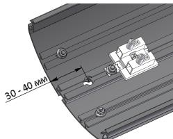
4. Set suspension systems at appropriate distance from each other. Minimum number of pendants needed for line assembly  $n = N+1$ , where  $n$  - number of pendants,  $N$  - number of luminaires in a line (one pendant in each joint of closed loop).
