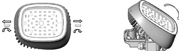
4. Insert the power wire into the housing through the sealed lead-in. Attach the luminaire to the mounting surface using the X3 mounting kit (not included in delivery kit) In case of using another mounting elements, the warranty for the luminaire is not valid.
