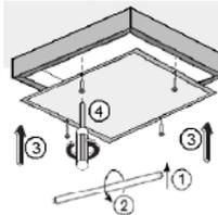
5.8. Luminaires installation should be done with X2 mounting hardware kit (doesn't included). Using of other mounting hardware will void the warranty.
