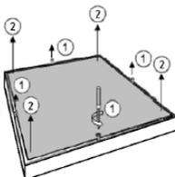
2. Put mains cable through sealing bush (included) which is inserted into appropriate opening in the luminaire's body.
