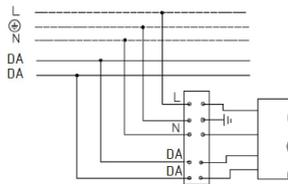
2. Mains connection scheme of luminaire with regulated control gear and ME6-NF unit.
