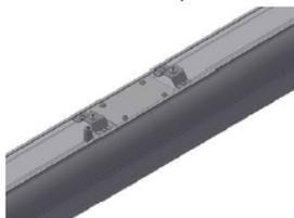
6. Fasten luminaries between each other with link (bringing luminaire right up to previous one) inside body.
