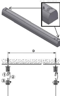
5. Insert joining bracket into slots and fasten it on top of luminaire (for line mounting of luminaire).
